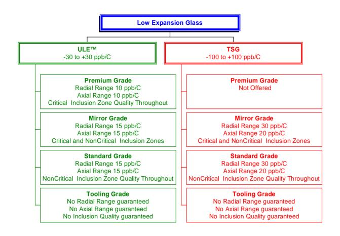
CTE values specified are for the Mean CTE from 5 to 35C Inclusion Zone Quality Specifications vary depending on size of blank
